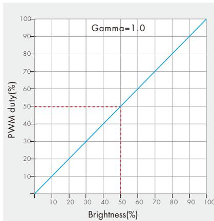
Dimming curve for RGB/DIM
